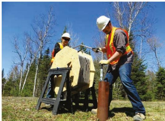
Figure 7.79 **Outil SAA (Measurand ShapeAccelArray)**
