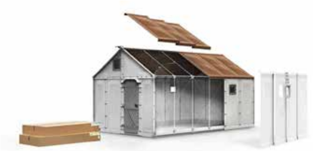
4. Principe constructif d'un abri Better Shelter, © Better Shelter.
