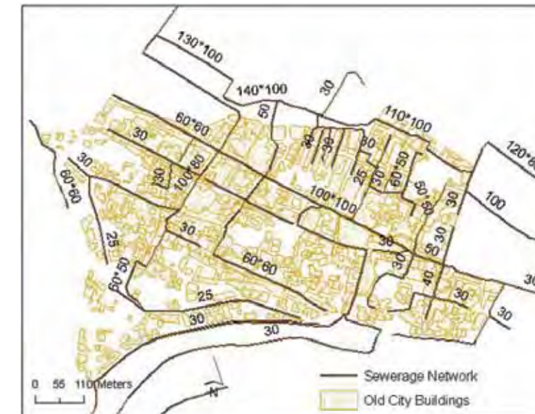
Figure 9.5 Sewage network of the Old City Source: Water and Sanitation Department in Nablus Municipality, 2009
